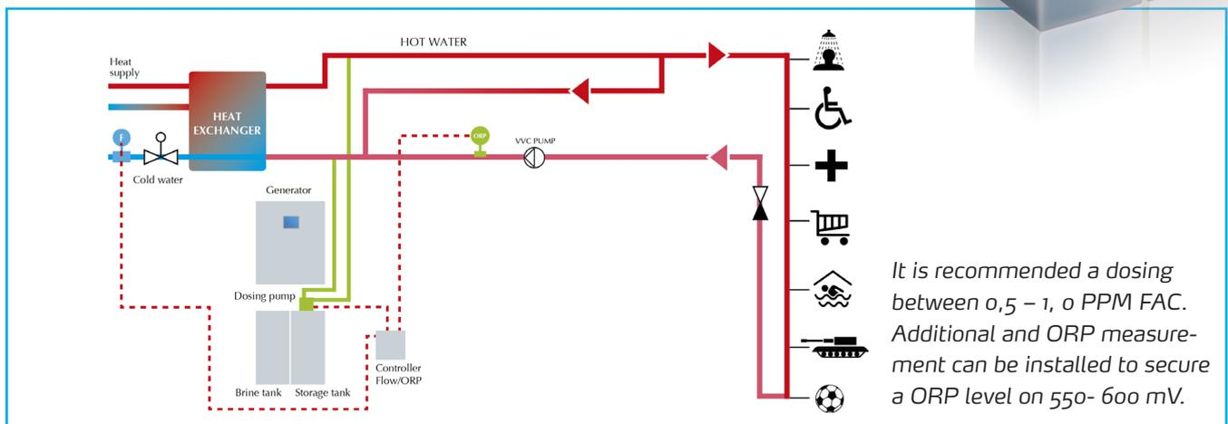
*It is recommended a dosing between 0,5 – 1, 0 PPM FAC. Additional and ORP measurement can be installed to secure a ORP level on 550- 600 mV.*
